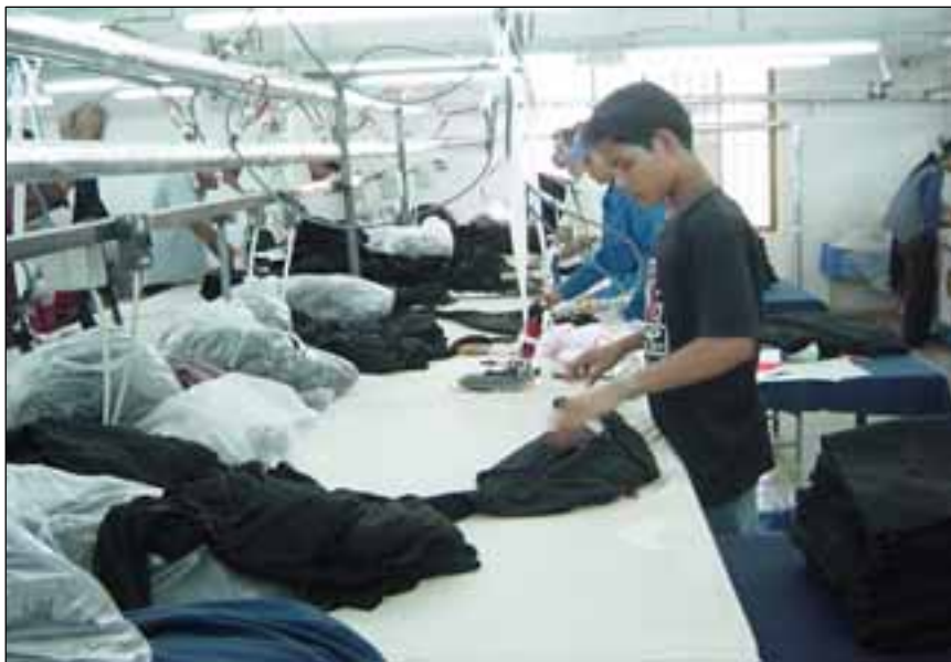
Picture 16: These workers are exposed to hot, humid conditions. Managers often try to reduce the temperature by placing fans around the workers or by introducing local exhaust ventilation systems that remove the hot air. The workers must also be provided with adequate drinking stations.
