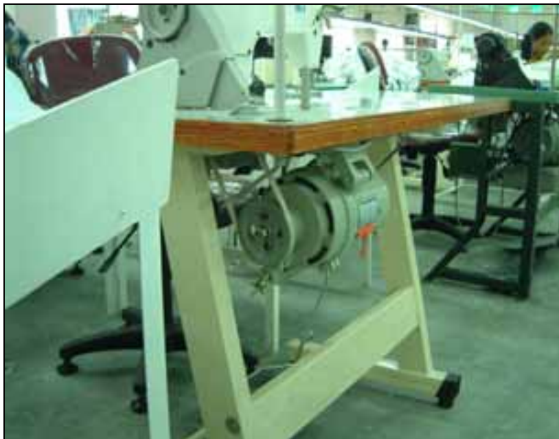
Pictures 5 and 6: Unguarded belts above and below the sewing table. It is easy for loose hair, clothes and necklaces etc. to get caught.
