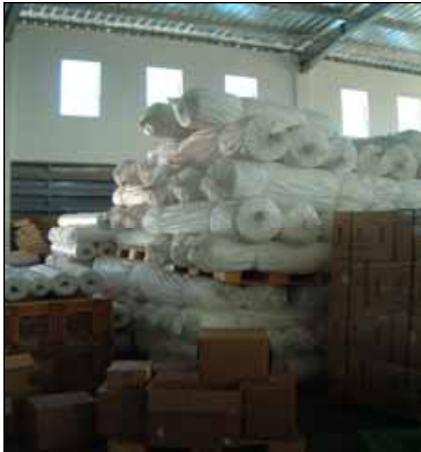
Picture 8: Poor stacking. The rolls of material could easily fall and cause injury.
