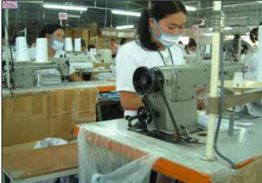
Picture 4: Unguarded machine in the weaving shed of a factory. Note that the machine is covered with dust, which also represents a hazard (see later).
