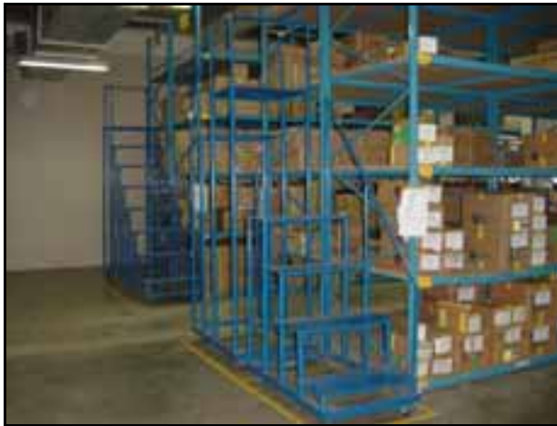
Picture 11: Use racks to store materials and finished goods.
