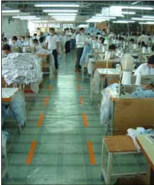
Picture 7: Clearly marked and unobstructed aisle.
