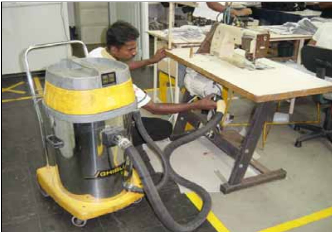
Picture 43: Look at this picture from a garment factory in Sri Lanka. This company uses an industrial vacuum to clean the machines and reduce dust levels in the workplace.
