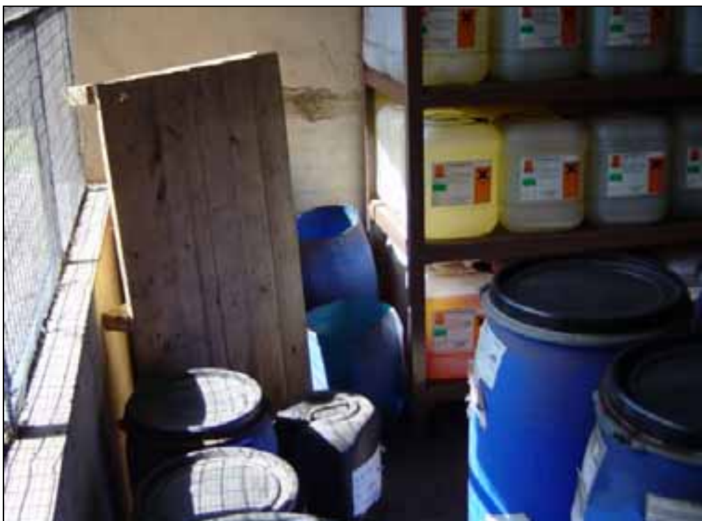
Picture 51: Look at these flammable chemicals being stored in direct sunlight.
