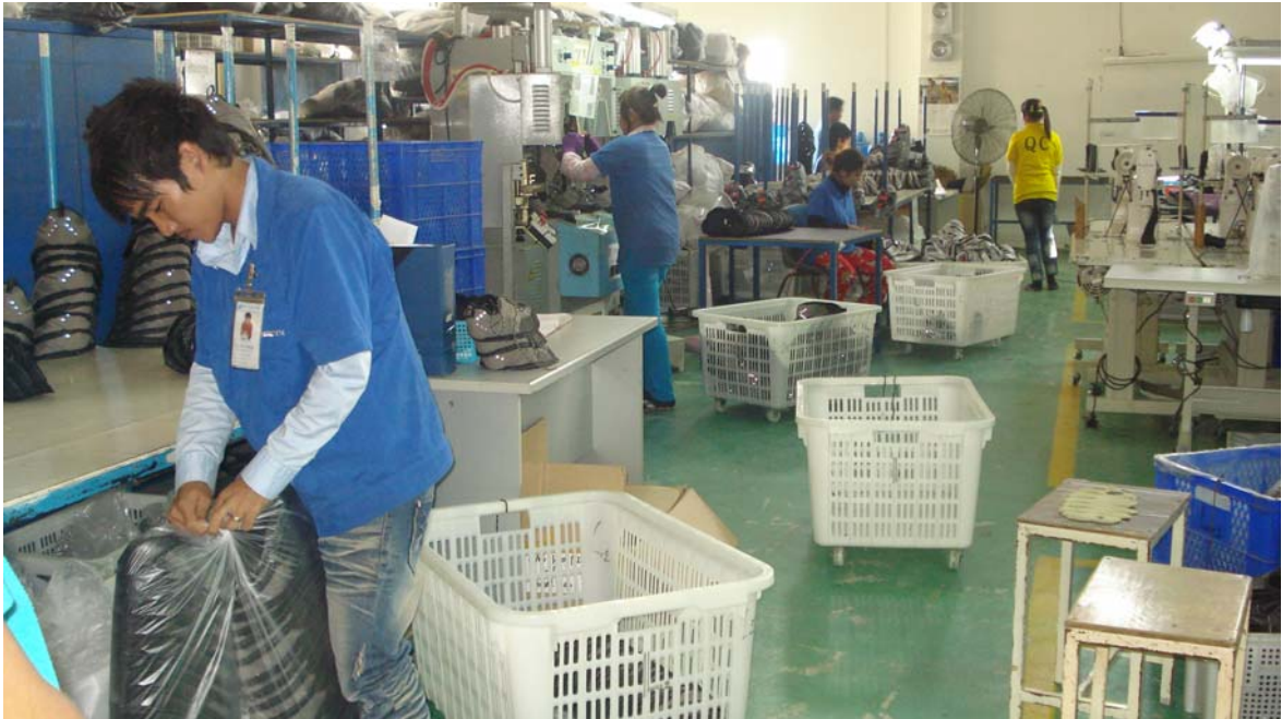
OSH Inspection: Access path (walkway) was blocked by materials and baskets.
